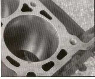
On top, the decks are likewise opened up to accept 1/2-inch ARP head studs (OEM is 11mm), and the cylinder bores are widened by 0.030 inches (about the limit of the 3.8's thin-wall construction) and finish-honed for moly rings.
