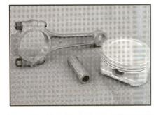
Tom strives to keep things affordable and one of the best ways to do this is to use factory parts whenever possible. His 4.4 reciprocating assembly combines 6.125-inch Chrysler rods with GM hypereutectic pistons as used in late-model super-charged Buicks (fly-cut, as necessary, for piston/valve clearance) rod bolts are replaced with ARP hardware. Of course, if you're planning a high-boost blower application and want custom rods and pistons, Morana can accommodate you.
