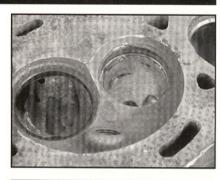
Alloy 3.8 heads are readily available in the scrapyard, so Tom likes to experiment. For instance, he got to wondering what would happen if you lowered the exhaust valve seat, as shown in this butchered trial version. In properly finished form, this experiment netted an additional 15–20 cfm. Is it something most people would bother with? Probably not, but this is the sort of thing that Tom just needs to know.
