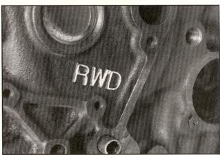
If searching the wrecking yards for a spare block, it's important to remember the 3.8 was also used extensively in front-wheel-drive applications like the Taurus. Though internally not much different than those found in a Mustang, FWD engines had different bell-housing bolt patterns and must therefore be avoided. Luckily they're easy to tell apart: the front of the blocks bear either RWD or FWD cast-in identification (Thunderbird Super Coupe blocks are marked "SC").
