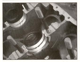
For the 4.4, Tom drills and taps the blocks for 1/2-inch ARP main studs, in place of the 11mm factory hardware. The stock main caps are then drilled to accommodate these larger studs. Though not yet done on the pictured block, the bottom of the cylinder bores also require some clearancing for the new crank/rod combination.
