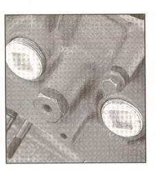
(Left) In one final modification, Morana prepares the block to receive screw-in frost plugs (as found in the old Boss 302), preventing any unexpected coolant departure, but also providing just a bit more block rigidity.
