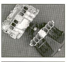
Another option for those needing maximum flow on the pre-split-port engines is to open up the intake combo to a rectangular port configuration, instead of the factory's oval shape.
