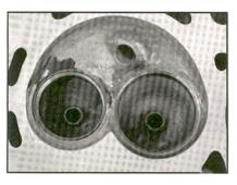
When it comes to valves, Morana likes to open the split-port's exhaust up to 1.65 inches (from the factory 1.45), but tends to leave the 1.86-inch intake valve alone. On the pre-'99 canted-valve heads, he can go as large as a 2.02/1.60 valve package, depending on application.
