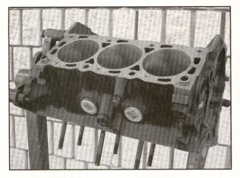
The starting point for a Morana Racing 4.4 stroker is an alignhoned and decked 3.8 block, preferably of '87 or newer vintage as these have a beefier bottom end and are configured for roller cams. Strongest of all are the ones fitted to the supercharged Thunderbird SC and Cougar XR-7, which wore gigantic main caps and steel cranks, but also had slightly different main journal diameter than run-of-the-mill 3.8s.
