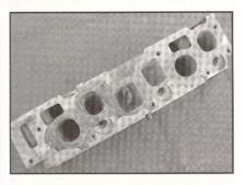
For any 3.8 variant, Morana offers both old-style and split-port heads ported to suit your requirements. On this split-port example, the two center intake ports have been opened up to flow over 280 cfm, in comparison to the as-yet-uncut outer ports, which Tom says flow about 170 cfm from the factory. When completed, this head will also improve from about 130 cfm on the exhaust side, to over 200 cfm.
