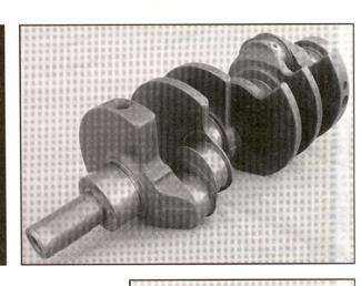
Normal 3.8 stroke is 3.390 inches. For his 4.4 stroker, Tom takes the cast-steel crank from the 4.2 truck engine (normally of 3.740-inch stroke) and offset-grinds it for a stroke of 3.925 inches. Another modification is widening the rod journal shoulders to accept a thicker rod. Normally internally balanced in the 4.2 engine, the assembly will be externally balanced when fitted to the 3.8 block.
